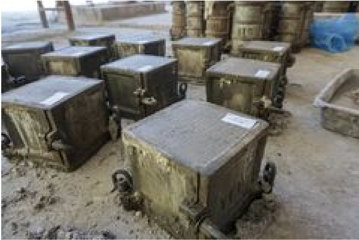
Figure3.2 Preparation of concrete cube
