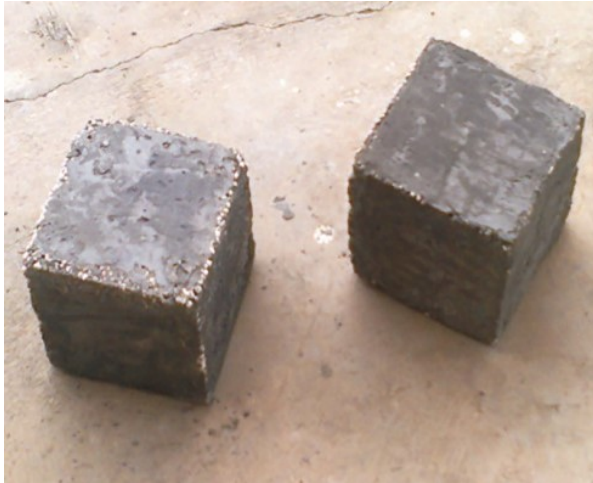
Figure3.3 Removed concrete cube
