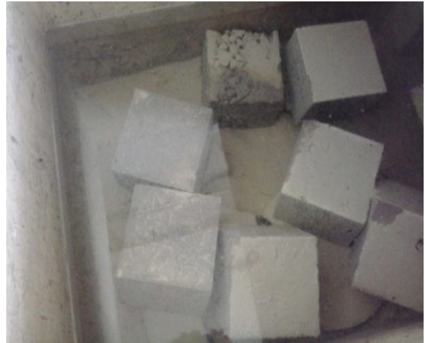
Figure 3.4 Curing of concrete cubes
