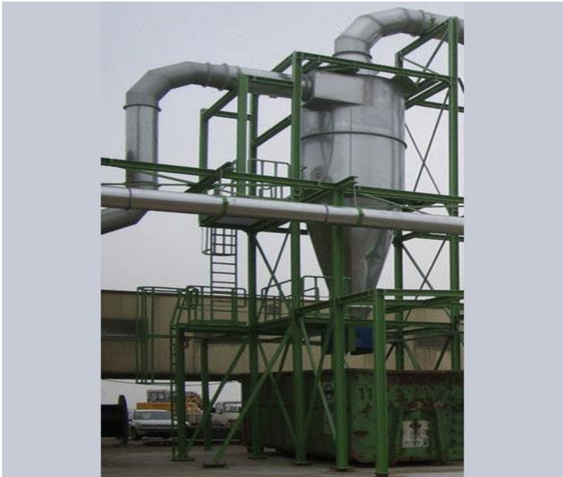
Figure 1.7: A Cyclone Separator installed in a factory (source: Google)
