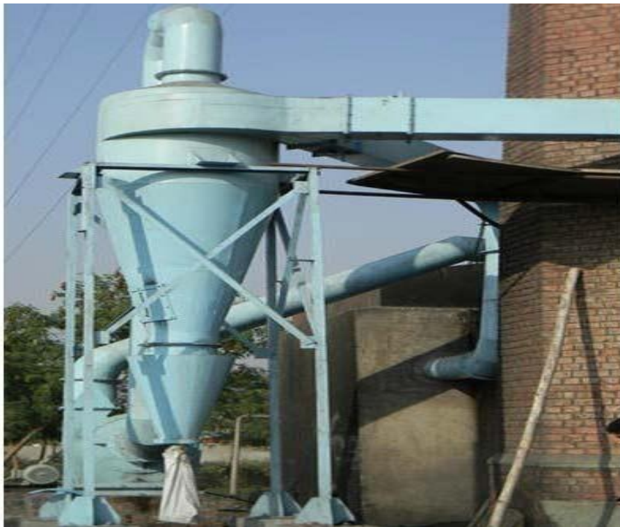
Figure1.6: Picture of Industrial cyclonic separator
