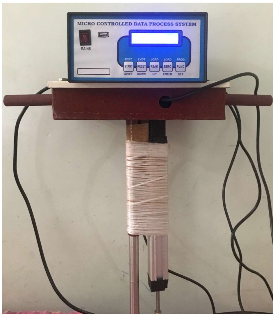
Fig. 3.3 Digital Static cone Penetrometer (Source: Present Study)
