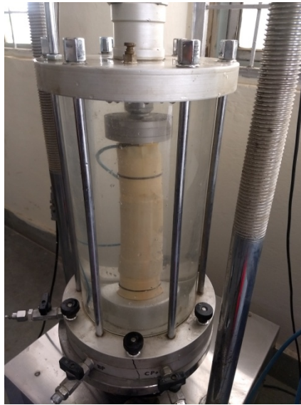
Fig. 4.12 UU Test performed at DTU Laboratory
