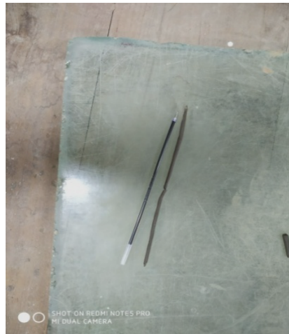
Fig. 3.4: Plastic limit test performed at DTU laboratory
