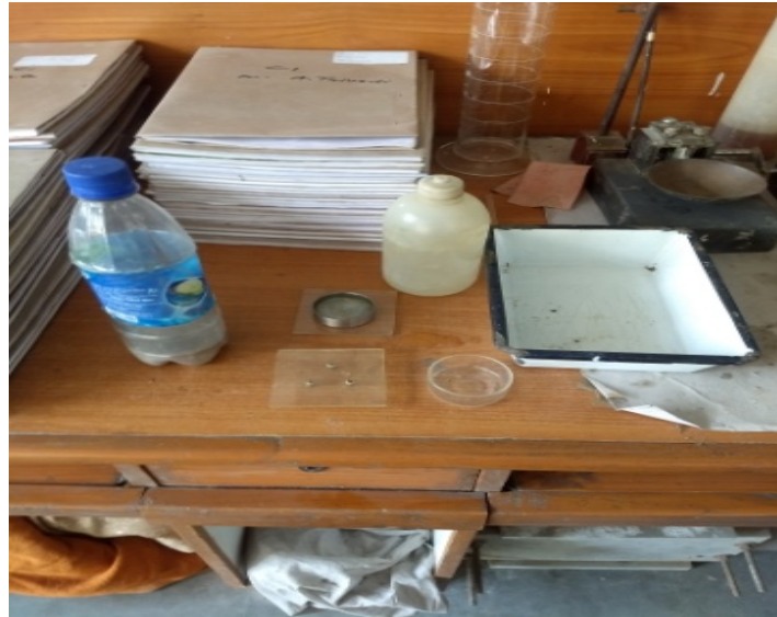
Fig. 3.6: Shrinkage limit test apparatus at DTU laboratory
