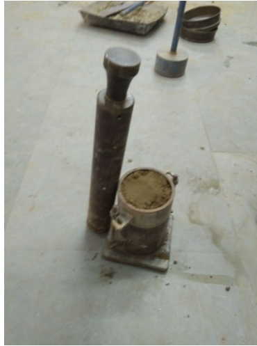
Fig. 3.9 Standard Proctor Test Apparatus at DTU Laboratory
