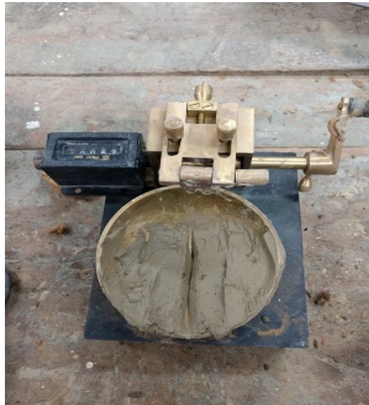
Fig. 3.5: Liquid limit test performed at DTU laboratory
