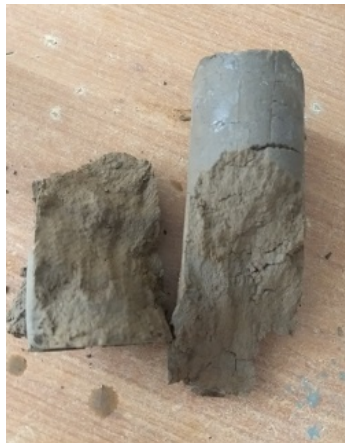
Fig. 4.16 Soil 3 after failure
