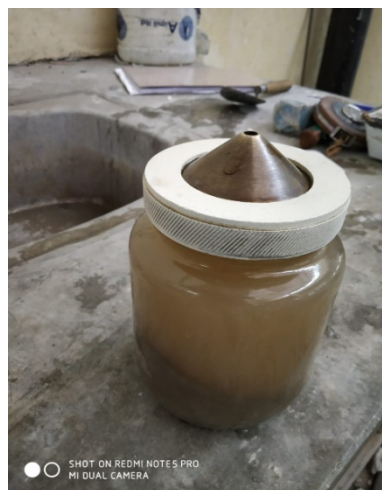
Fig. 3.7: Pycnometer used for the determination of specific gravity
