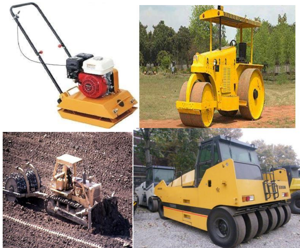
Fig 2.1 Various types of mechanical compactors a.) Vibratory roller b.) Smooth wheel roller c.) Sheep foot roller d.) Pneumatic tyre roller
