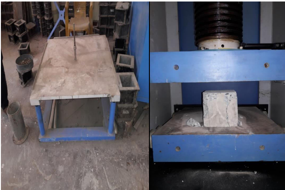
Fig 6.4 Compression testing machine and vibrator in concrete laboratory
