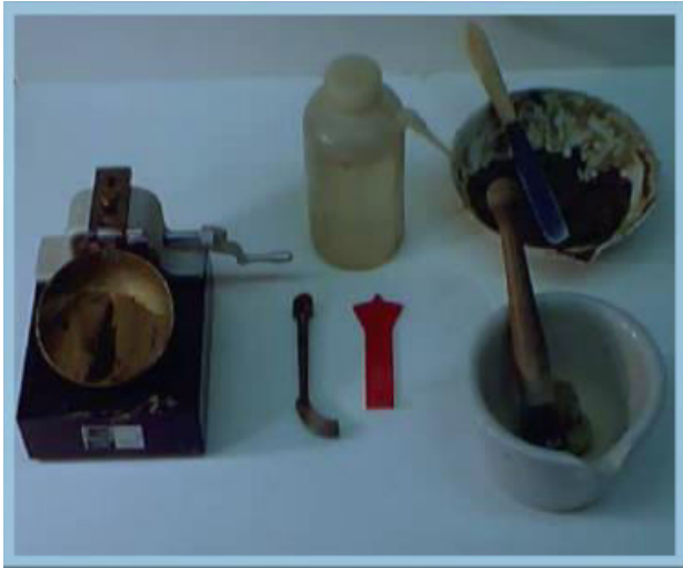
Fig 3.1 Liquid Limit apparatus with grooving tool
