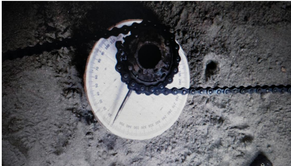
Fig. 3.10 Calculation of angle of twist
