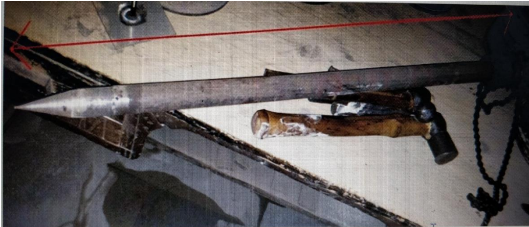
Fig. 3.3 Mild steel modal pile of 90cm length{DTU thesis}[4]
