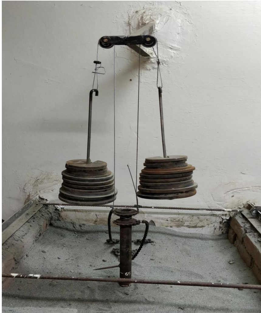
Fig.3.8 Full set up of Pull out test
