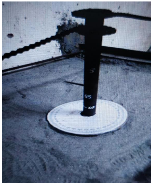
Fig. 4.3 Pile inside the Yamuna sand up to depth 55 cm
