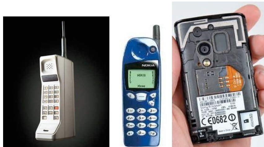
Fig. 1.1 (a) The Motorola DynaTAC with a monopole antenna.(b) The Nokia 5510 with a helical antenna (c) The Sony Ericsson Xperia with the patch antennas visible at the top
