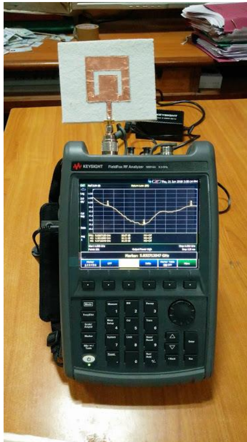
Fig.5.10 Measured result of S11 parameter
