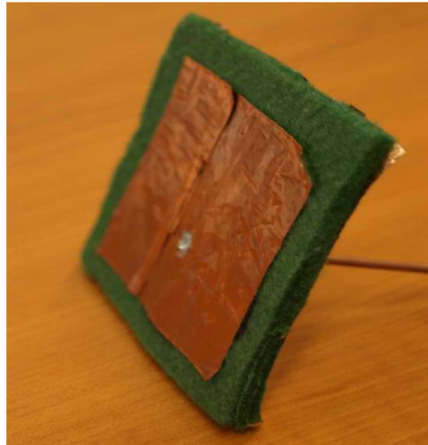
Fig.3.4 Peeled off copper tape due to environmental conditions [39]
