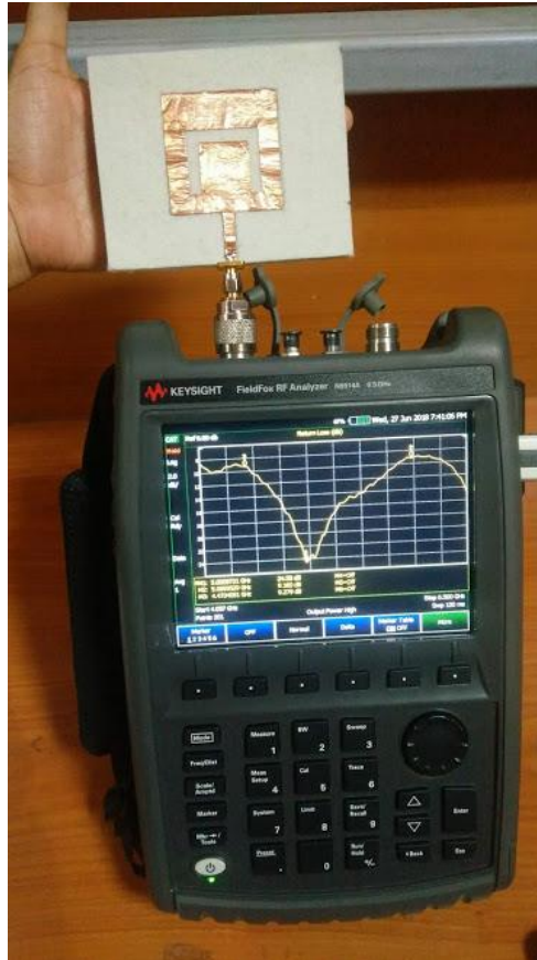
Fig.5.11 Measured result of S11 parameter in the presence of body
