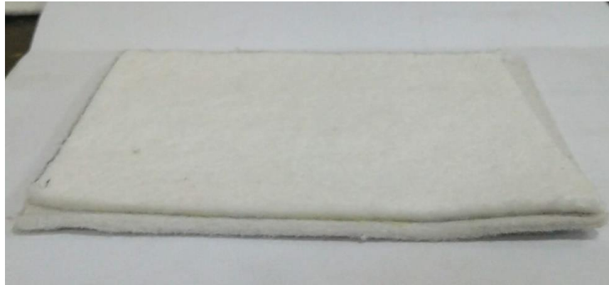
Fig.4.8 Two layers of felt are stuck together using glue
