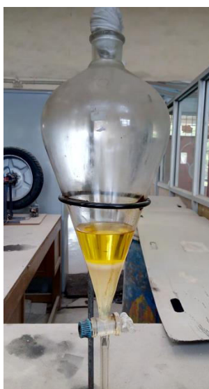
Figure 4.12: Separating flask with water washed biodiesel sample (upper layer biodiesel and lower layer water-catalyst mixture)
