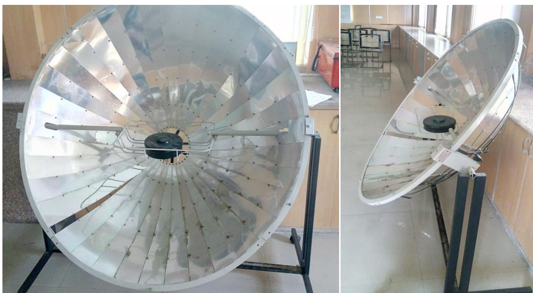
Figure 4.3: Front and Side view of paraboloid solar dish collector with receiver
