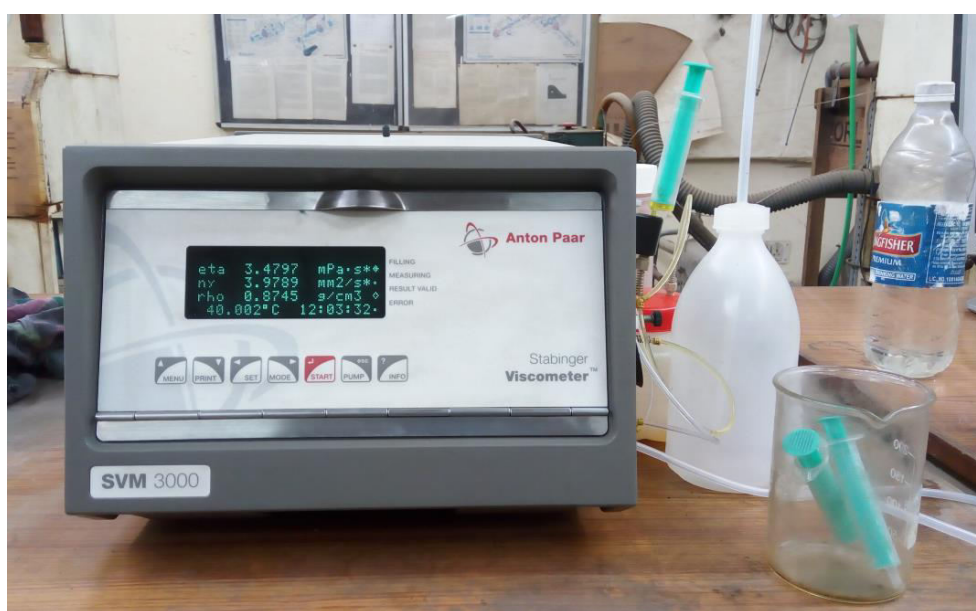
Figure 4.8: Viscometer used to measure kinematic viscosity and density of samples
