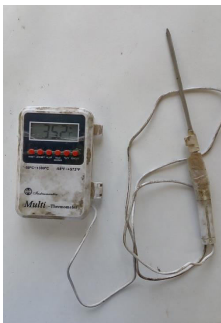
Figure 4.7: Thermocouple used to measure sample temperature
