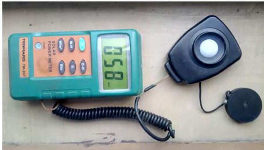
Figure 4.1: Solar power meter with solar intensity sensor
