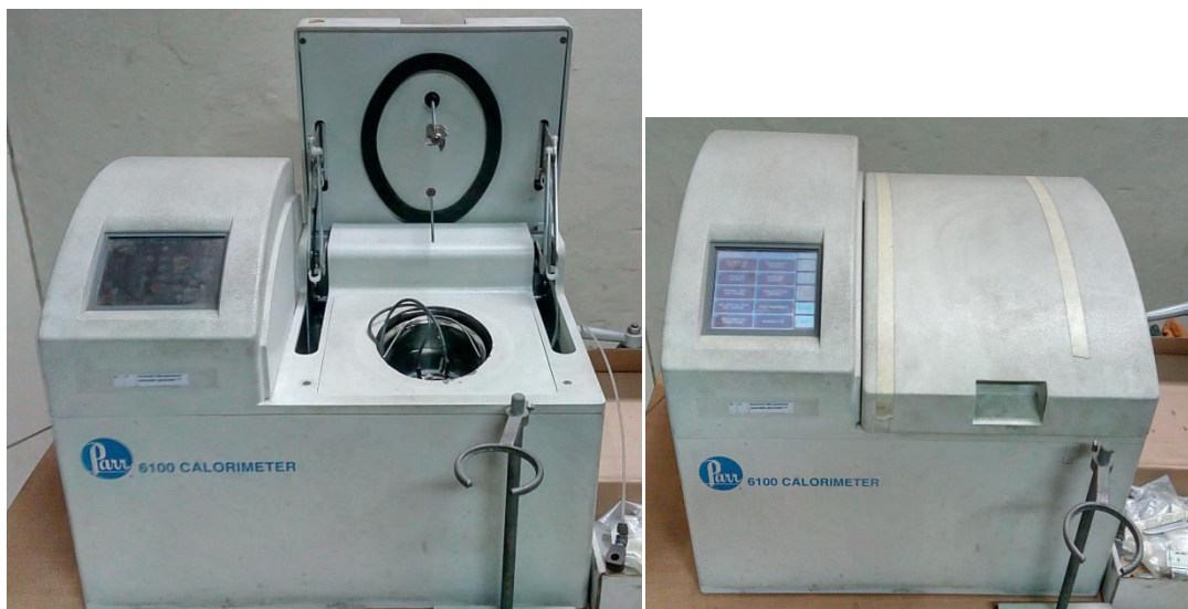
Figure 4.9: Calorimeter used to measure calorific values of biodiesel sample
