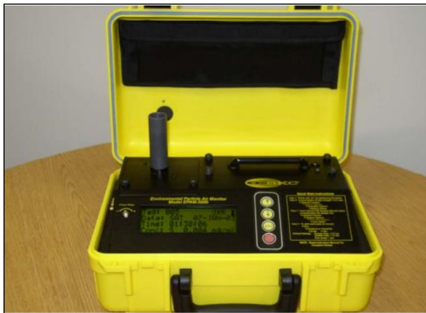
Fig.3.2 EPAM5000 haz Dust
