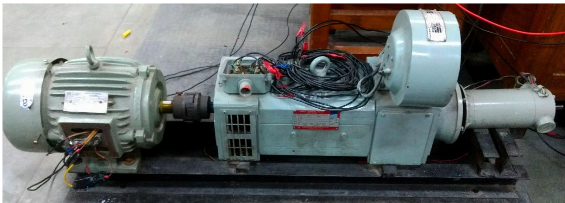
Figure 5.4 Induction Motor Coupled with DC generator and Tachogenerator
