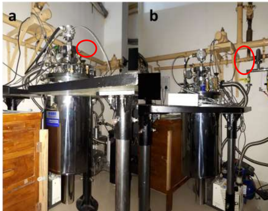
Fig.3.7: Connection of bellow with (a) helium reservoir at one end and with (b) helium recovery line at another end.
