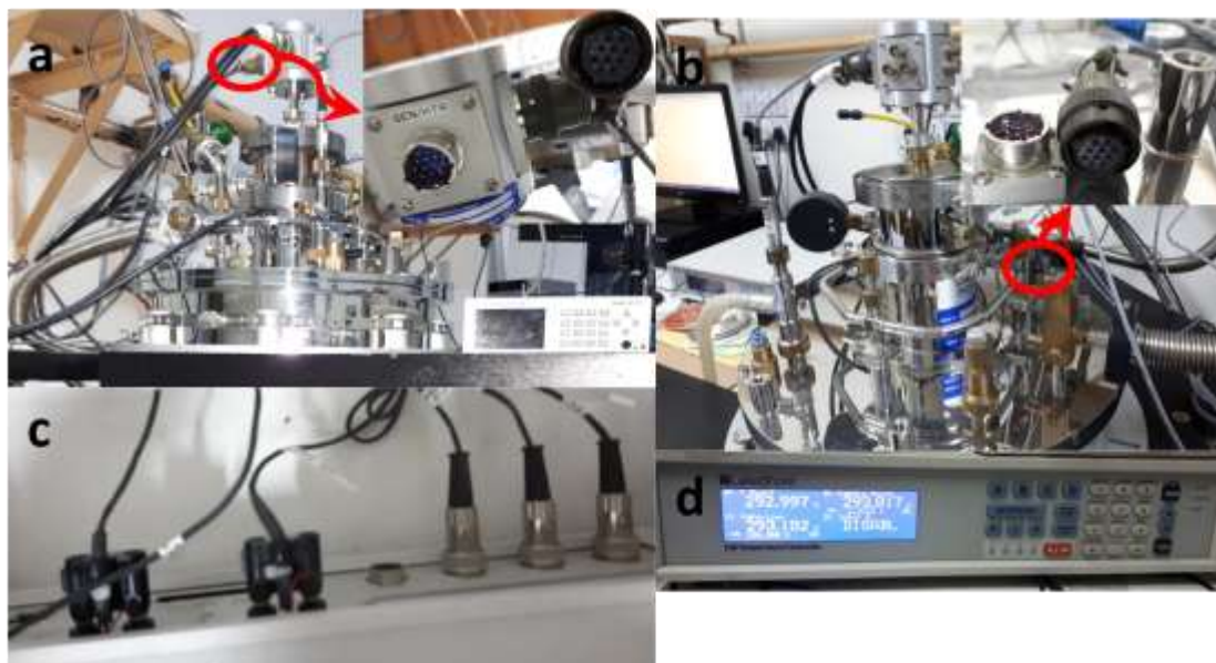
Fig.3.2: 10 pin feed through for connection with temperature sensor and heater from (a) sample space and T-mount in probe (inset zoomed view) as well as (b) vaporizer and its connection with temperature controller (inset zoomed view) (c) back view showing three sensor connection (sample space, T-mount, vaporizer) and two heater connection respectively from right (d) front view showing temperature at sample space, T-mount, vaporizer and fourth sensor is not connected.
