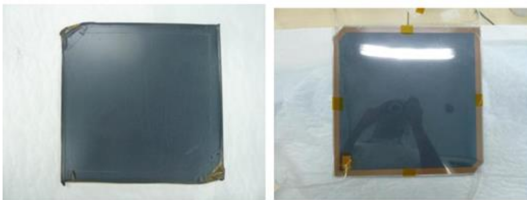
Figure 4.9 Pictures of RPC after painting with graphite paint and covering the surfaces with Mylar sheets.
