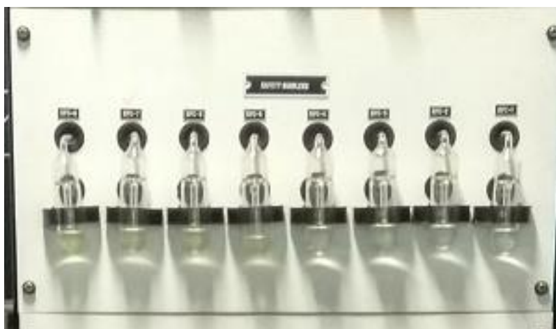
Figure 4.13 Safety bubblers showing no bubble implies that the chamber is leak free.
