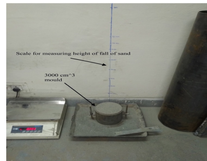
Fig. 3.4 Apparatus for the height of fall vs relative density
