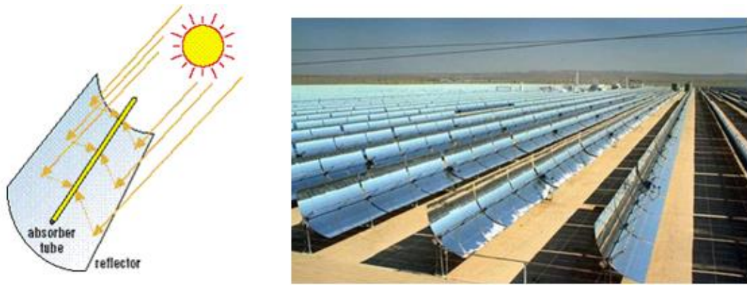
Figure 6: Parabolic trough technology principle (left)[5] and SEGS parabolic trough plant in California (right)[6]
