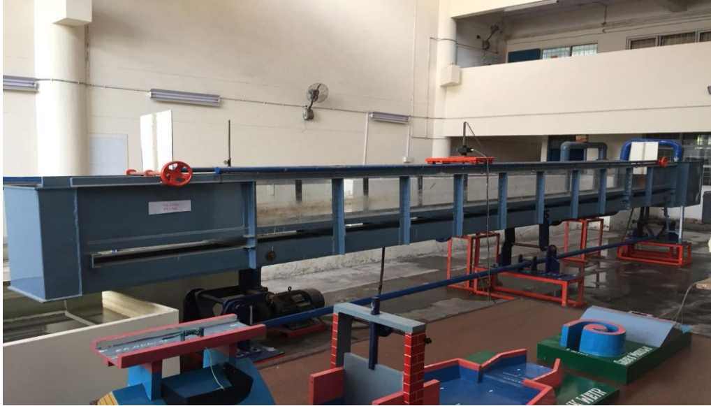
Fig 4.2 8 meter long Tilting flume
