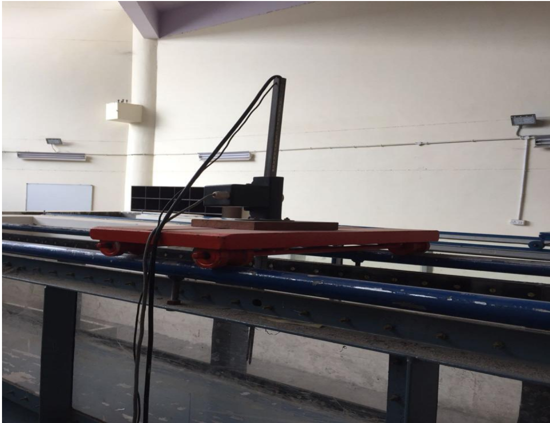
Fig 4.5 Measuring the Reading by using Point gauge
