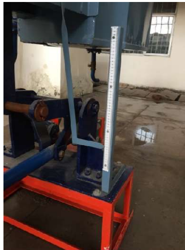
Fig 3.7. Scale showing height difference between upstream and downstream end of the flume
