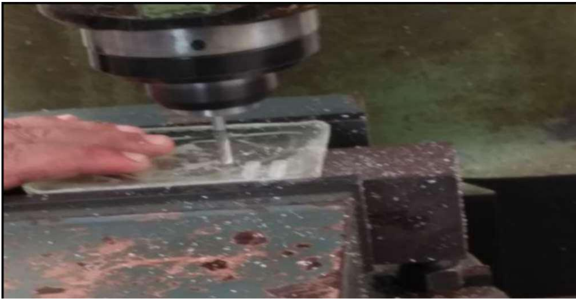
Figure 3.5: Machining on the neat sample
