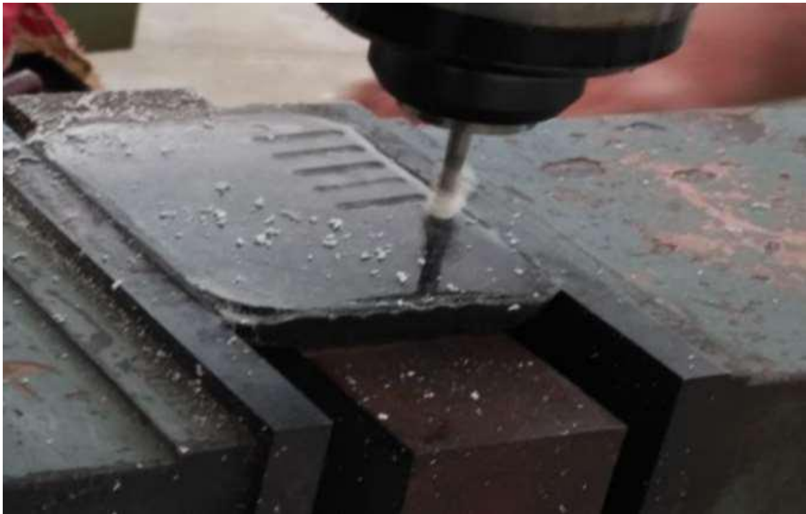
Figure 3.6: Machining on the GO-epoxy sample
