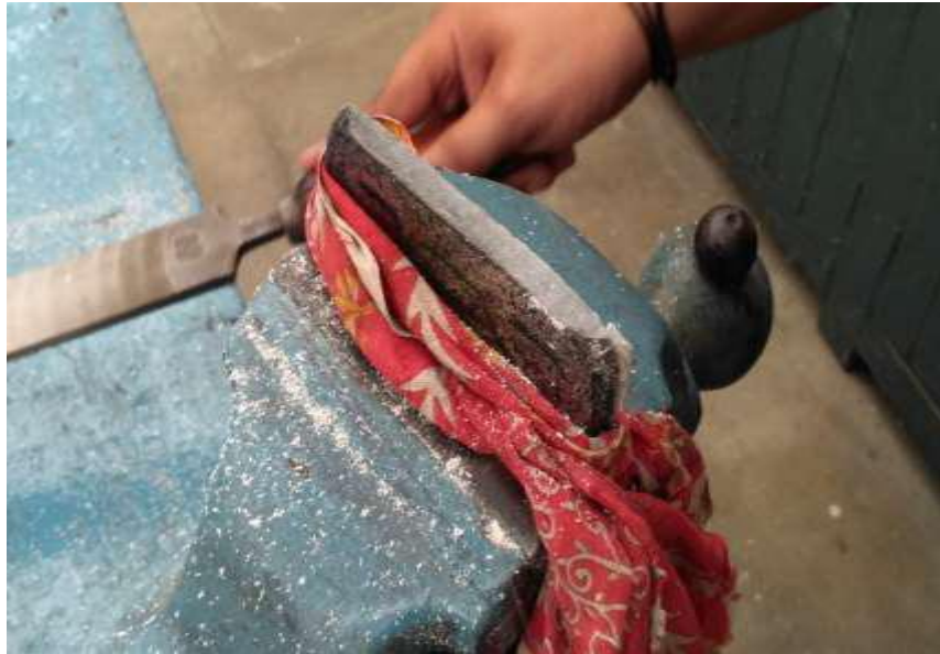
Fig 3.4: Preparing a sample for the milling machine
