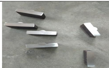
Figure :4.7 Weld bead after wet polishing
