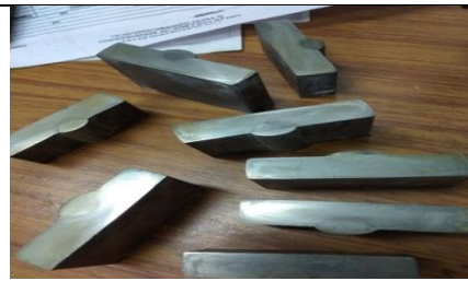
Figure: 4.8 weld bead after etching
