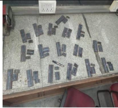
Figure 4.4 : specimen after cut by power hacksaw
