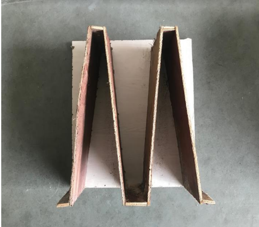
Figure 4.6. 8° labyrinth spillway model
