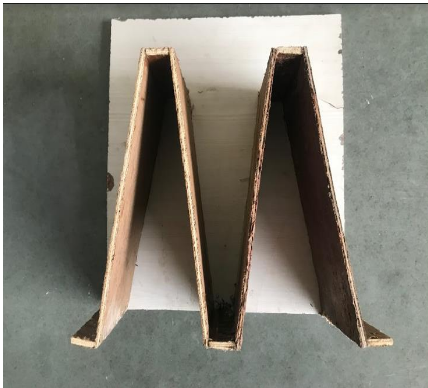
Figure 4.7. 10° labyrinth spillway model
