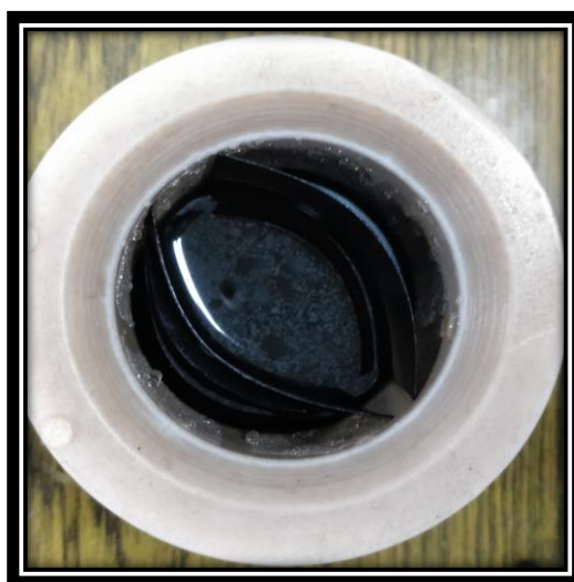
Figure: 5.3 Whatman filter paper after hydrothermal reaction
