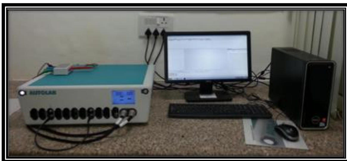
Figure: 4.6 Autolab Galvanostat/Potentiostat Instrument (Metrohm, The Netherlands)
