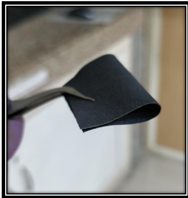
Figure 6.16 : Optical image of MoS 2 /Paper immunoelectrode showing flexible nature
