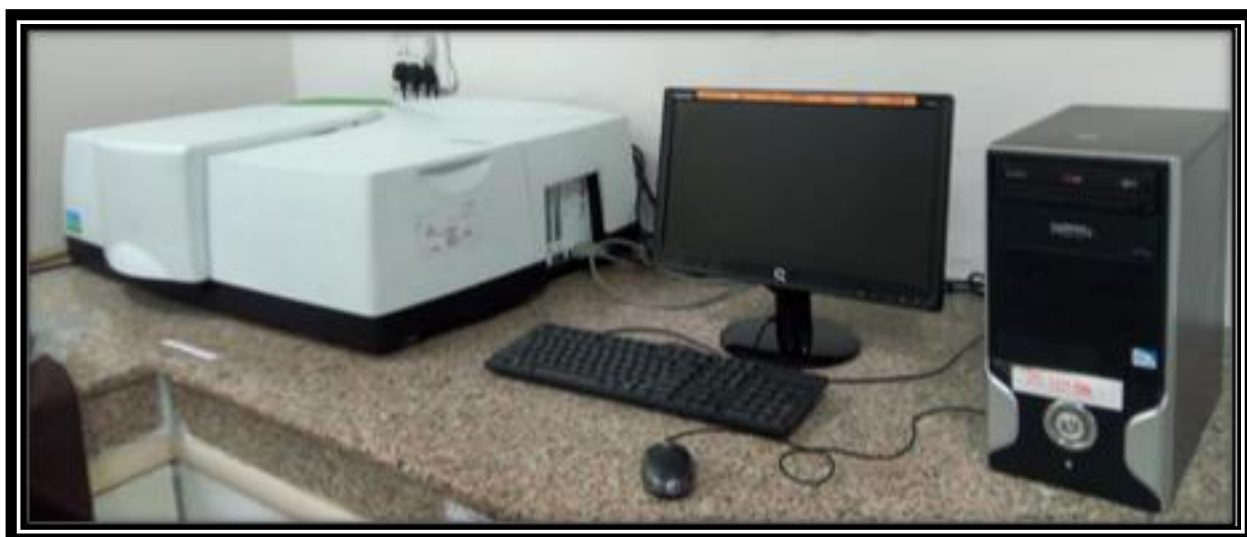
Figure 4.3: UV/Vis/NIR Spectrophotometer instrument (Perkin Elmer Lambda 950) SEP
