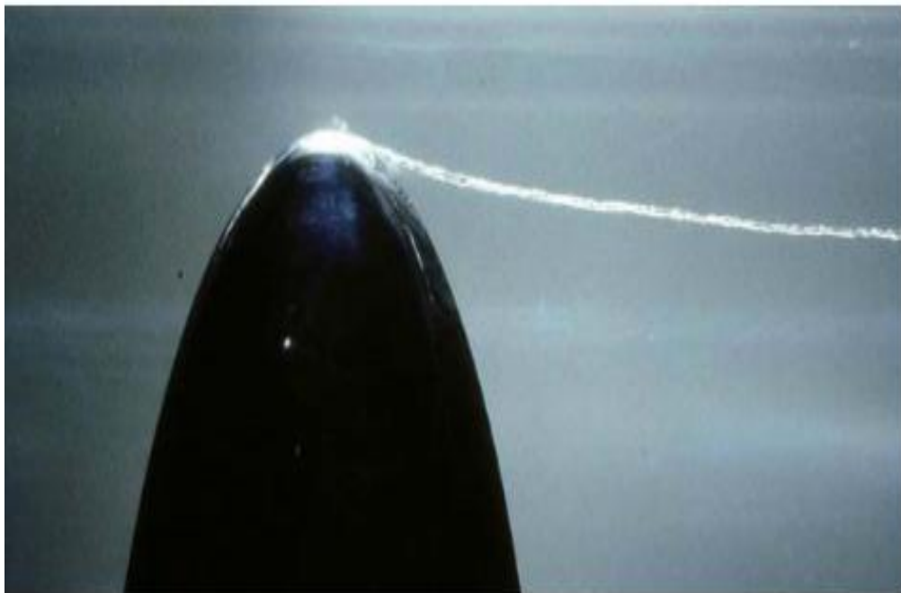
FIGURE 2.5: VORTEX CAVITATION GENERATED BY A THREE DIMENSIONAL HYDROFOIL
