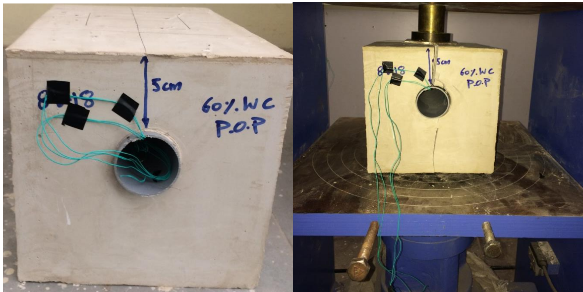
Figure 5.4.2 5cm cover depth before and after loading
