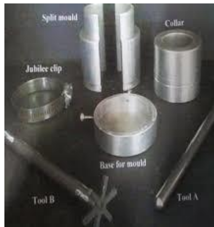
Figure 3.2 Unconfined Compression Test sampler
