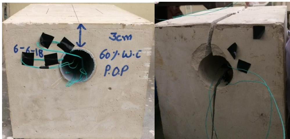
Figure 5.3.2 3cm cover depth before and after loading
