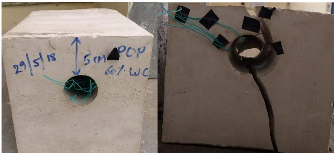
Figure 5.2.2 5cm cover depth before and after loading
