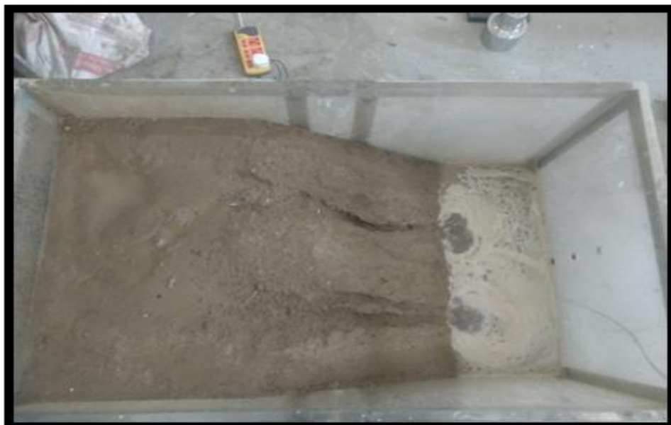
Fig. 6.6: Effect of rainfall at 40 mm (top view)
