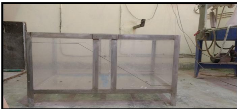
Fig. 4.2: Frame type box with marking on it according to Jhakri slope
