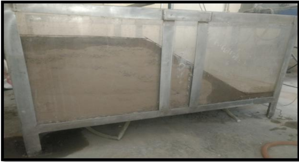
Fig. 6.3: Effect of rainfall at 30 mm depth (side view)
