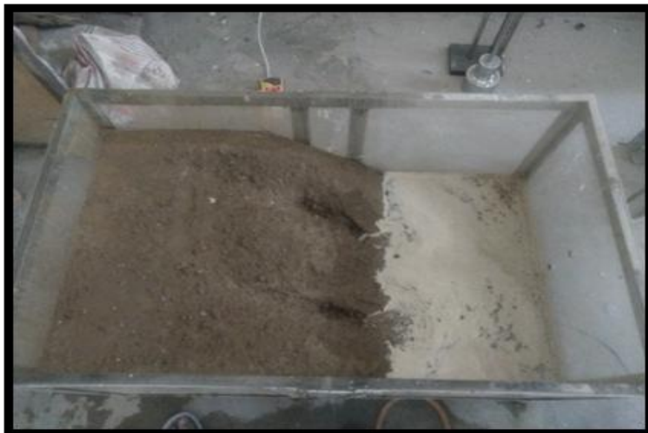
Fig. 6.10: Effect of rainfall at 60 mm depth (top view)
