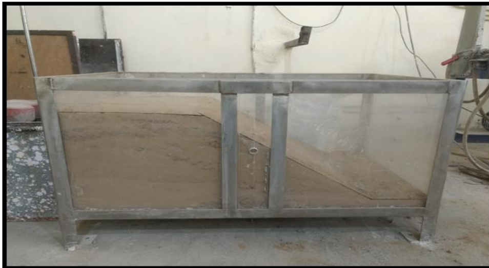
Fig. 4.3: Frame type model with soil slope
