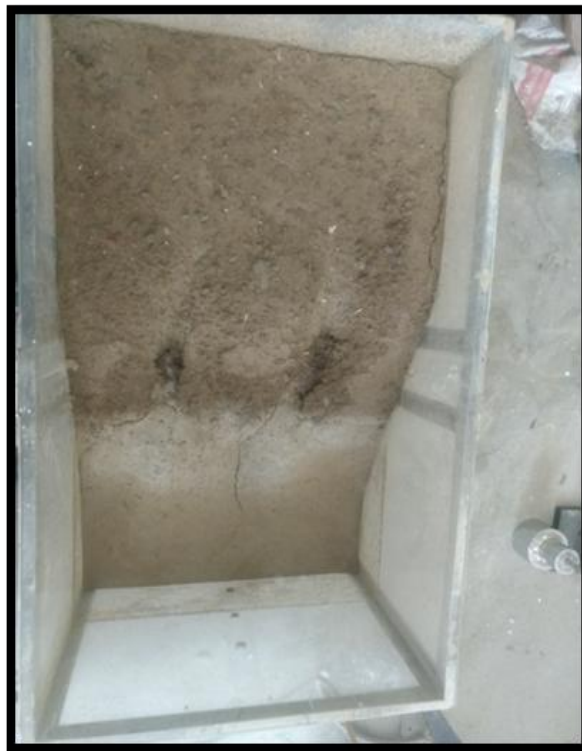
Fig. 6.12: Effect of rainfall at 70 mm depth (top view)
