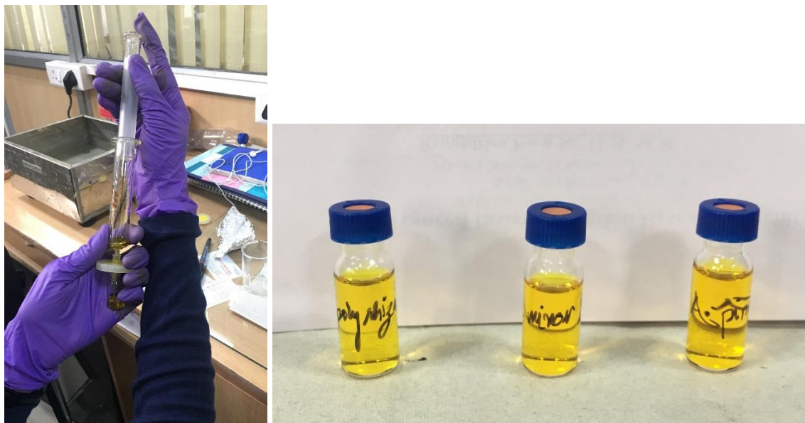
Fig 19: Filtering of sterol sample through 0.2 micron nylon filter (left), Final sterol samples in GC glass vials (right).
