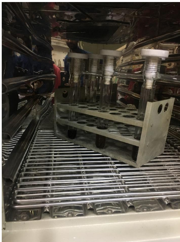
Fig 18: Digester tubes containing sample and acid in incubator
