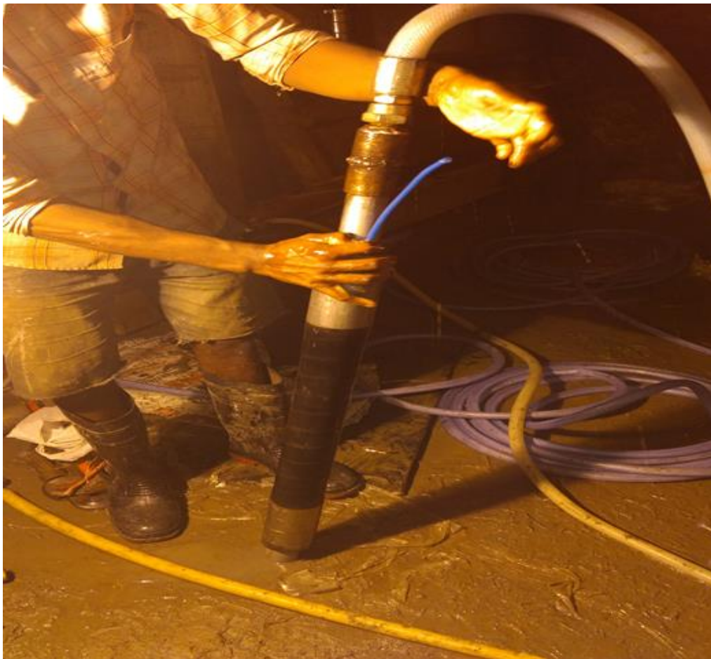
Fig 3.25 Lugeon values test with pneumatic packer.
