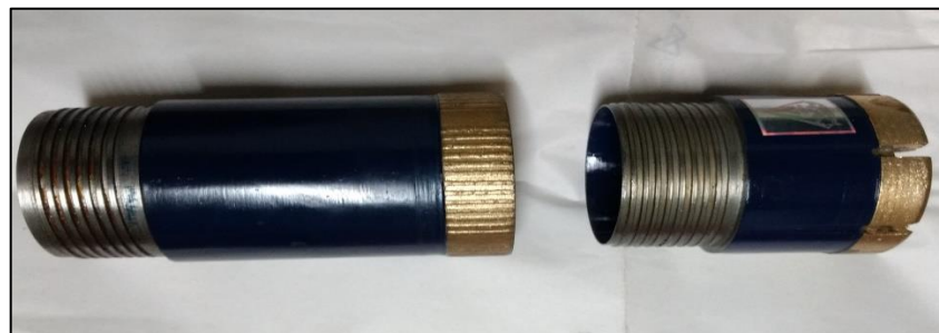
Fig 3.5 Drilling barrel and diamond drilling core bit.
