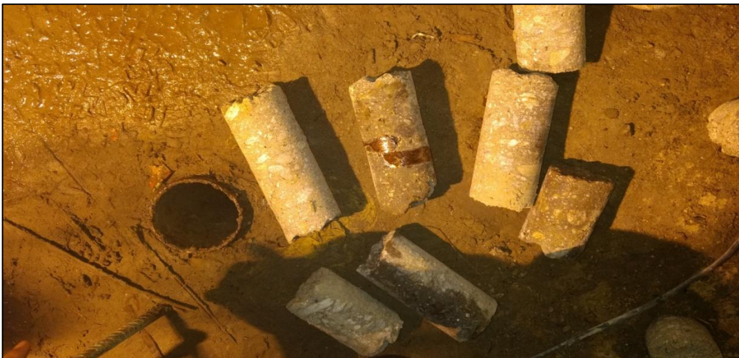
Fig 3.1 Casing embedded in the concrete section and core recovery of concrete
