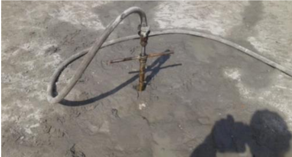
Fig 3.24 Lugeon values test with mechanical packer.
