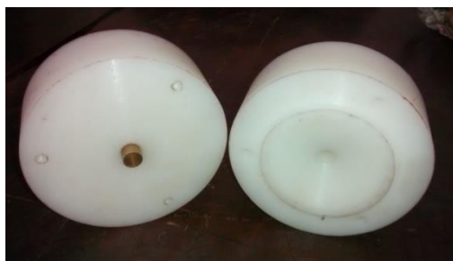
Figure 14. Nylon Fixtures used in AFM setup
