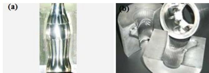
Figure 17. New glass moulds (dies and moulds)[9]
