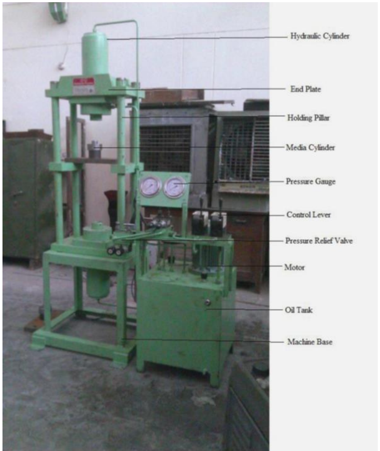
Figure 15. Vertical double acting AFM machine setup
