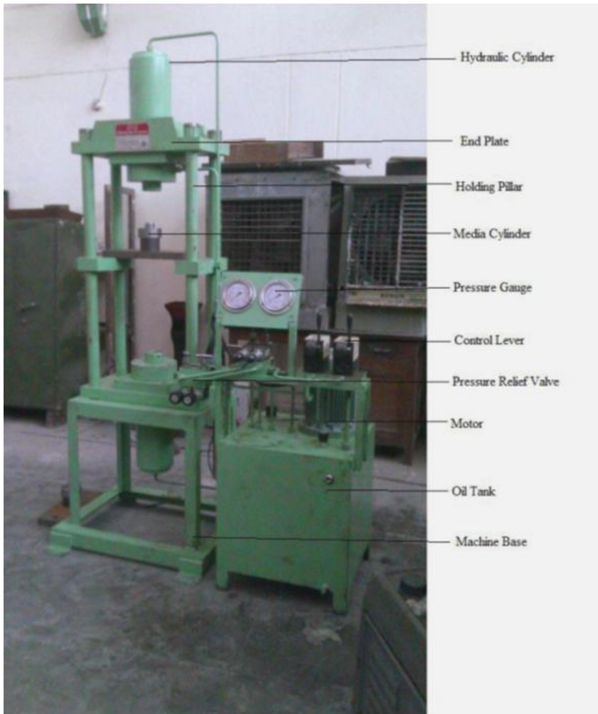
Figure 15. Vertical double acting AFM machine setup
