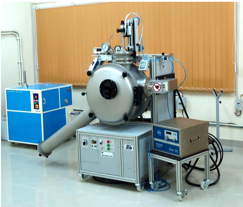
Figure 3.4. (a) Melt Spinning Unit (Make: Edmund Buhler GmbH, Model: Melt Spinner HV) used for synthesizing nanostructured ribbons/flakes (b) Water cooled Copper wheel with crucible
