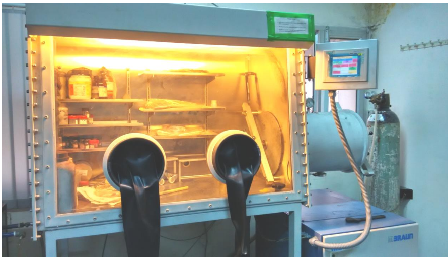
Figure 3.2. Glove box used for loading and unloading of ball milled powders from the Stainless-Steel Jars (Make: Mbraun, Germany, Model: MB20)
