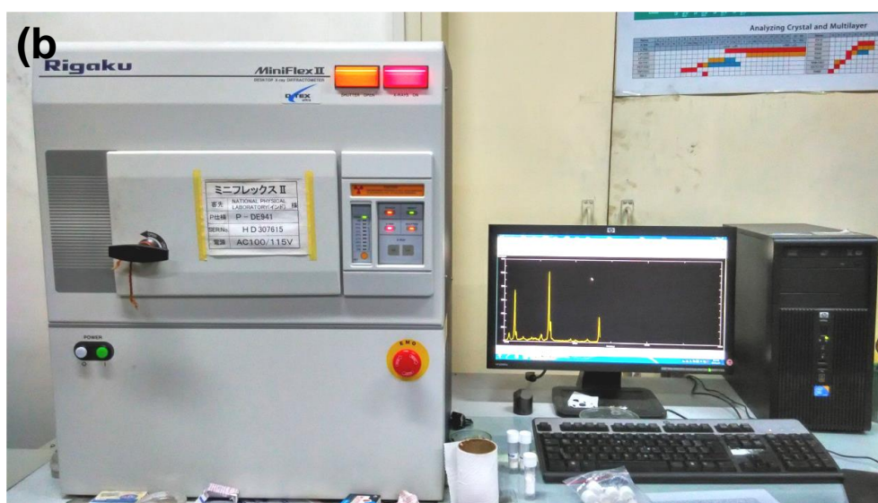
Figure 3.6. (a) Basic principles of X-ray diffraction and Bragg's law, (b) X-Ray Diffractometer used for characterization of crystal structure and phase purity of synthesized materials (Rigaku, Japan, Model- Miniflex-II)
