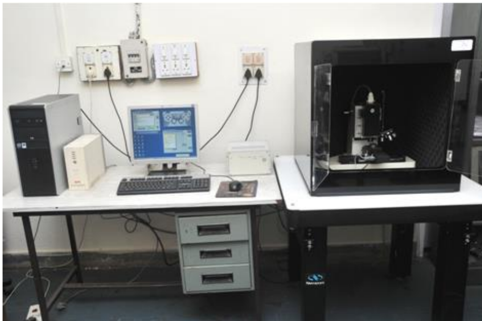
Figure 3.16. Nanoindentation equipment (Fischer-Cripps, Model: IBIS-B, Australia) used for Nanomechanical properties measurement.
