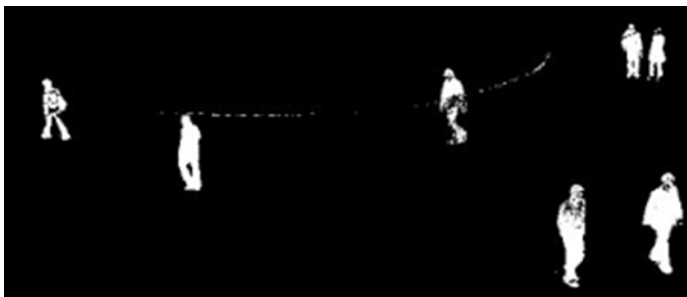
Figure 4.2: output after frame difference
