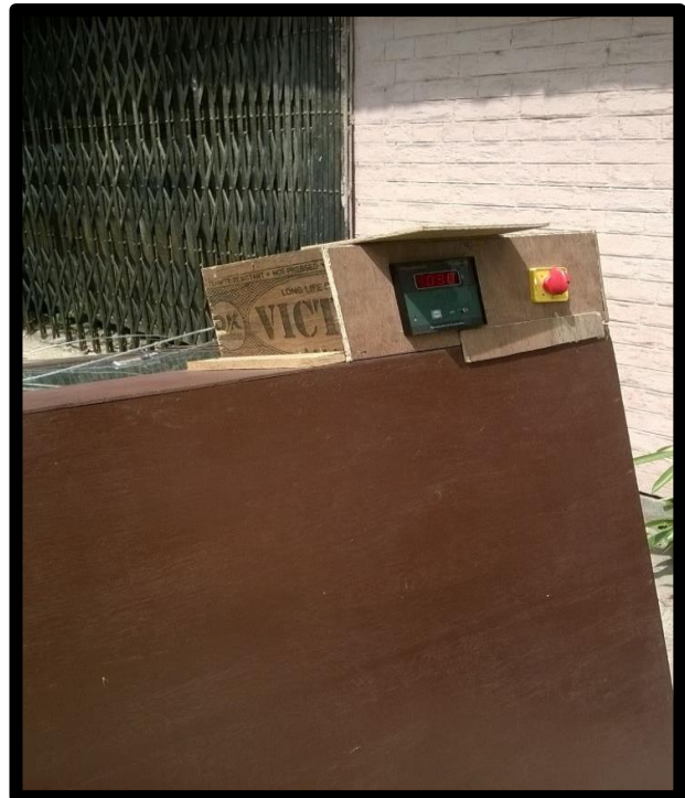
Fig. 3.20 Instrumentation (a) Locating surface thermocouples on drum (b) Output on digital display unit.
