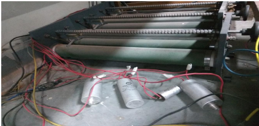
Fig. 3.19 Development of resistive capacitive (R-C) ripple filters
