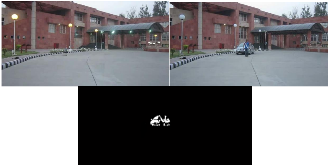
Fig. 3.8 (a) The Background, (b) The Current Frame and (c) The Foreground Mask
