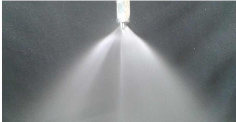
Figure 3.5 Water spray coming out from impaction pin nozzle
