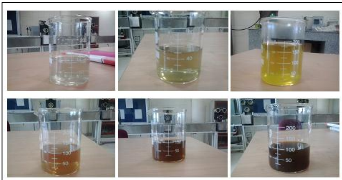
Figure 5.2.6(b): Change in colour with time due to the formation of silver nanoparticles
