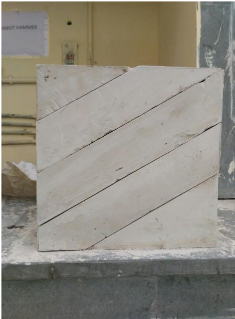
Fig- 3.6 (a): Prepared rock mass samples after cutting.
