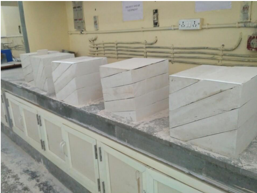
Fig- 3.6 (b): Prepared rock mass samples after cutting.
