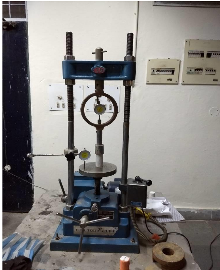
Fig-3.3: Unconfined compression test.
