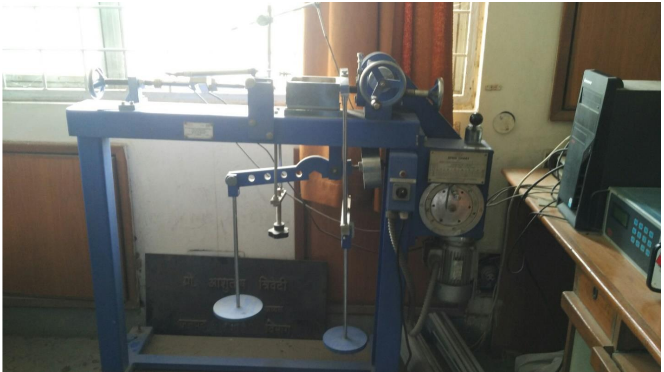
Fig-3.1: Direct Shear Test apparatus
