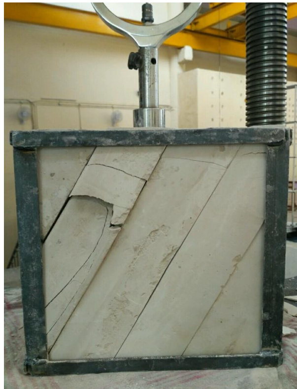
Fig- 3.12: Sample with joint orientation 60^\circ (After failure)
