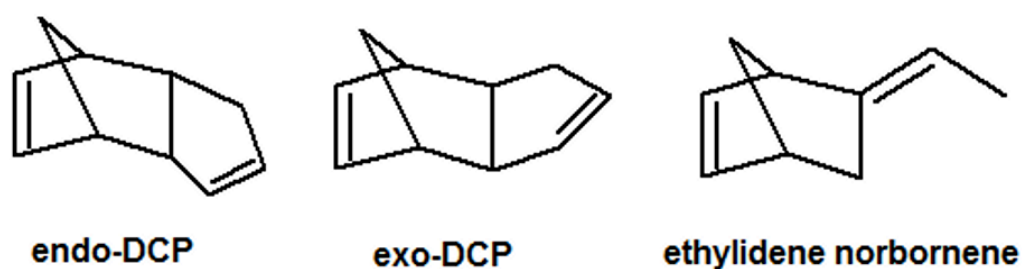
Figure 1.7: Monomers capable of undergoing ROMP, showing potential as healing agent
