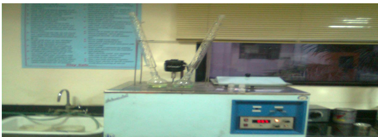
Figure A1.6: Water bath with Air Condenser
