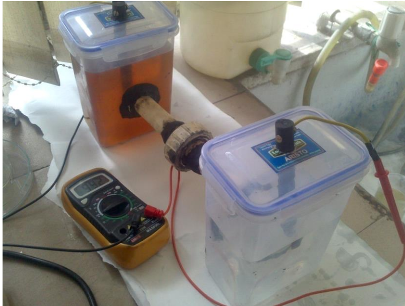
Figure 10: Two membrane setup with PEM configuration and no use of mediator in the medium
