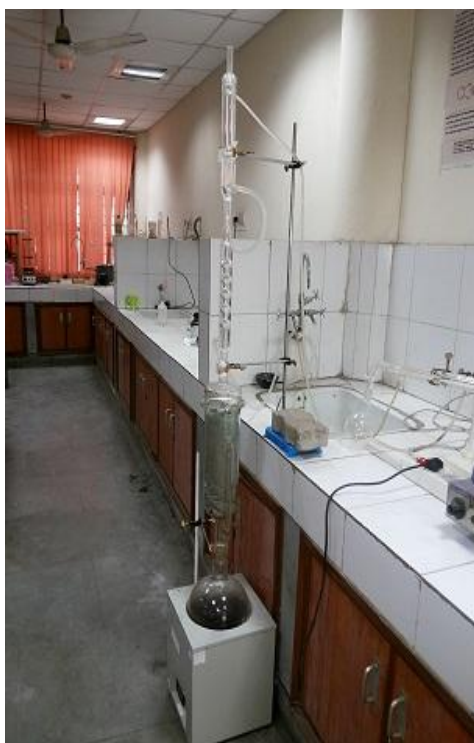
Figure 5.3: Soxhlet extractor with flower of B. ceiba
