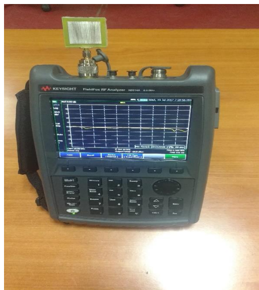
Fig 5.9 VNA measurement of fabricated antenna
