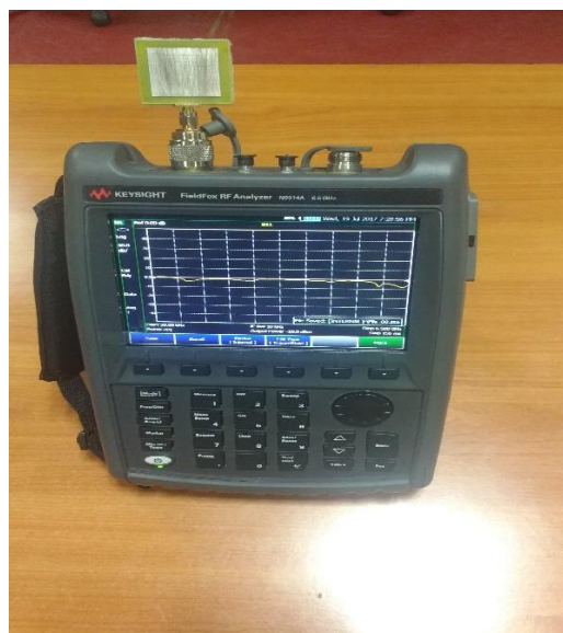
Fig 5.9 VNA measurement of fabricated antenna
