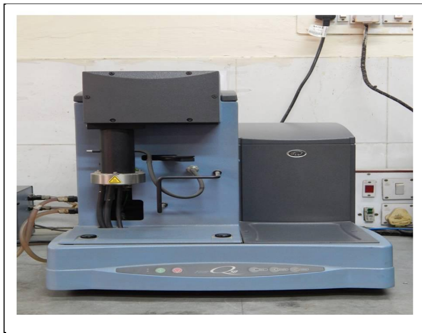
Figure AP-2.2: Thermogravimetric analysis (Universal V4.5A, TA Instruments)
