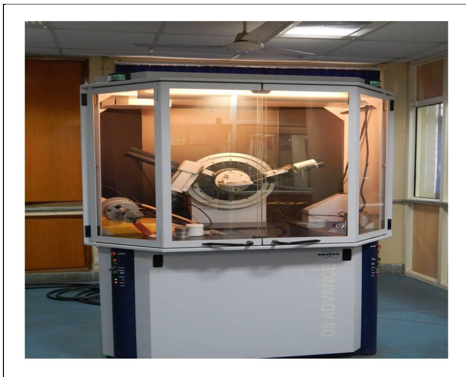
Figure AP-2.3: X-ray diffraction (D-8 Advance, Bruker)
