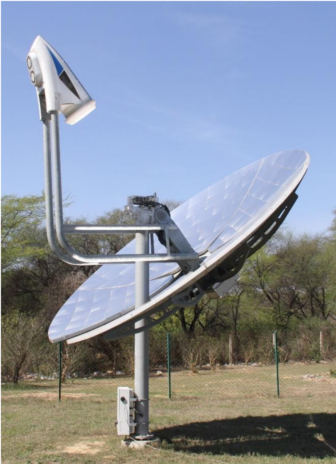
Figure 2.6 Paraboloid dish concentrators with stirling engine installed at NISE.
