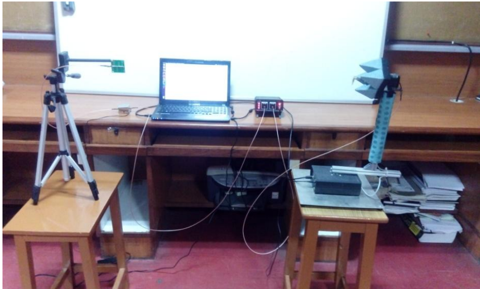
Fig. 5.13 Antenna measurement using Anechoic Chamber prototype
