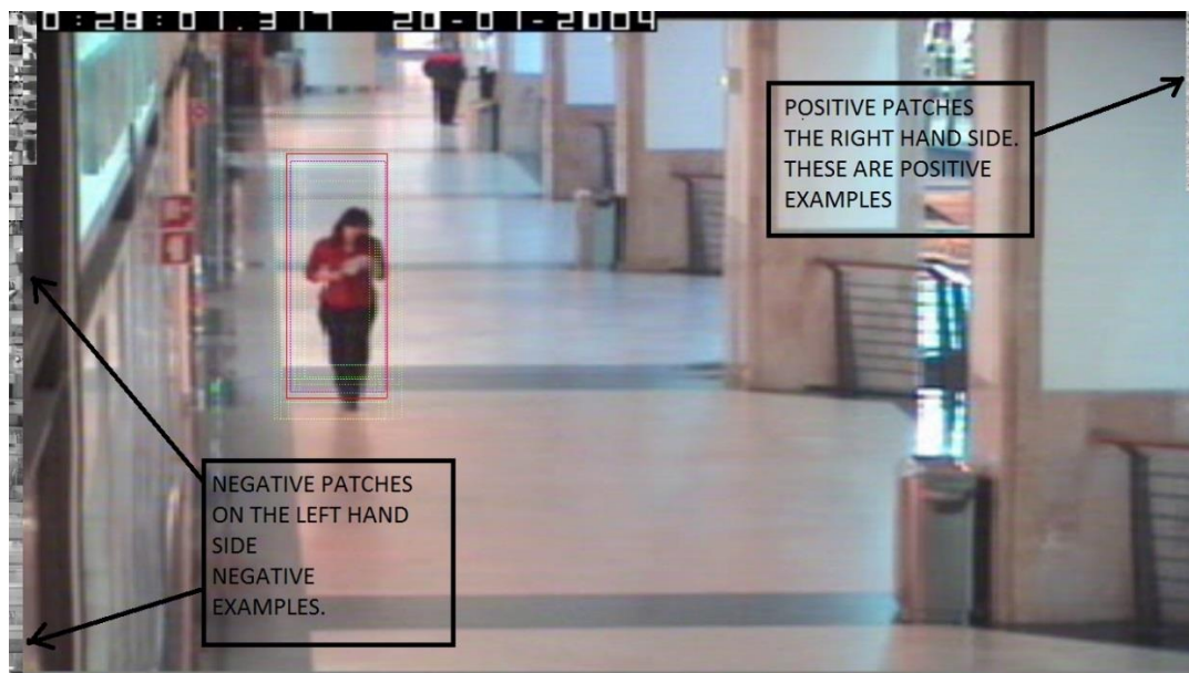
Figure- 6.10 Frame showing positive and negative patches in right and left side.
