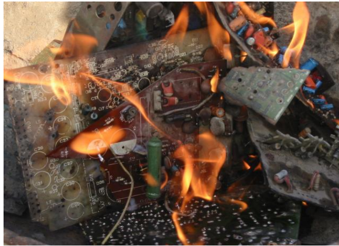
Figure 2: E-waste (PCBs) being incinerated in open environment
