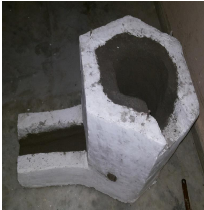
Figure 15: Concrete cell of plasma pyrolysis reactor
