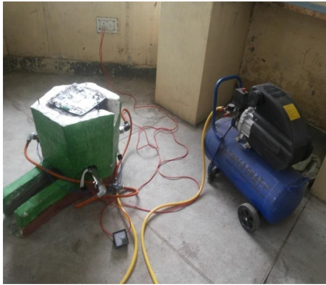
Figure 23: Plasma pyrolysis reactor set up
