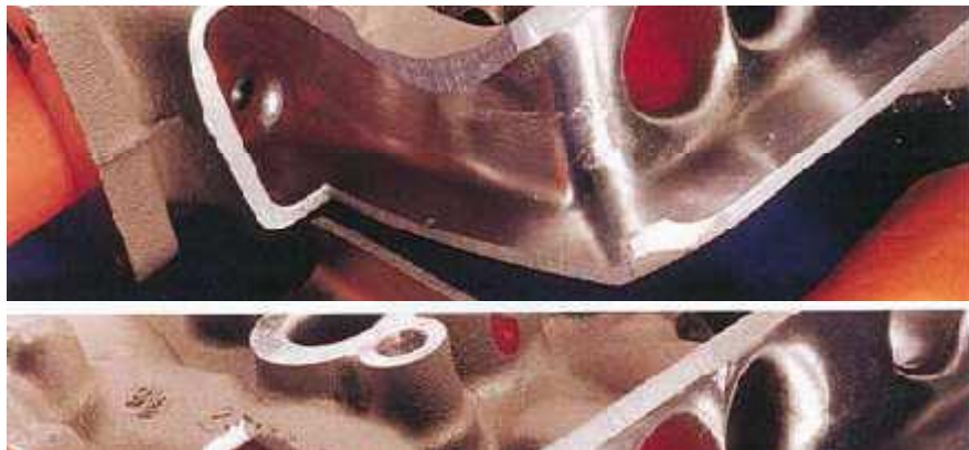
Figure 6: Intake manifold after manual AFM processing [9]
