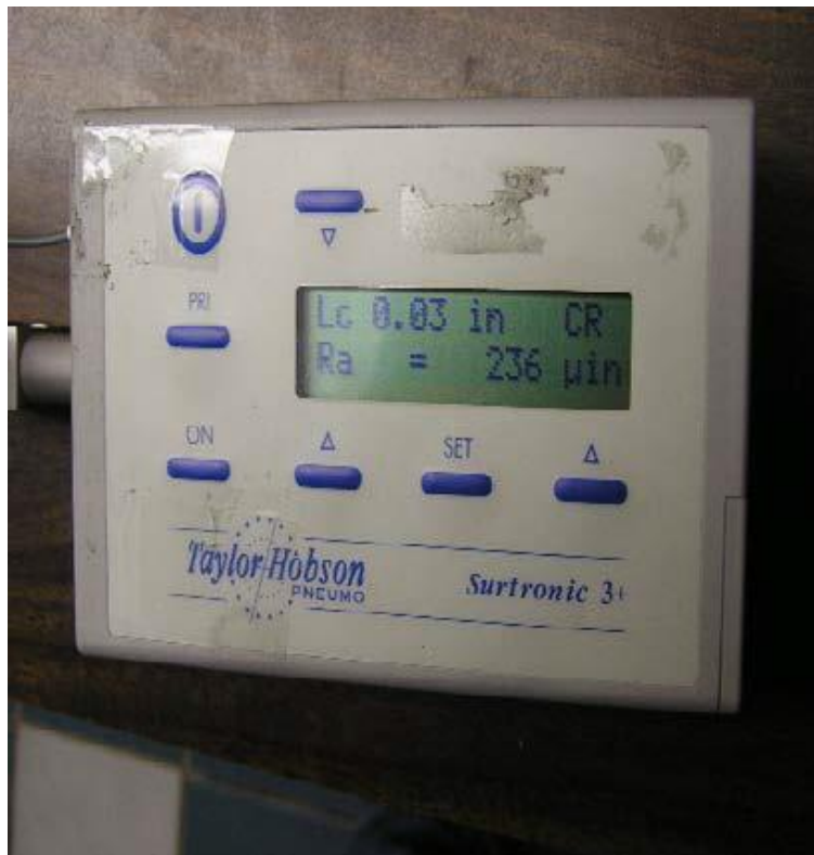
Figure 11: A talysurf instrument by Taylor Hobson Surtronic 3+ at metrology lab, DTU
