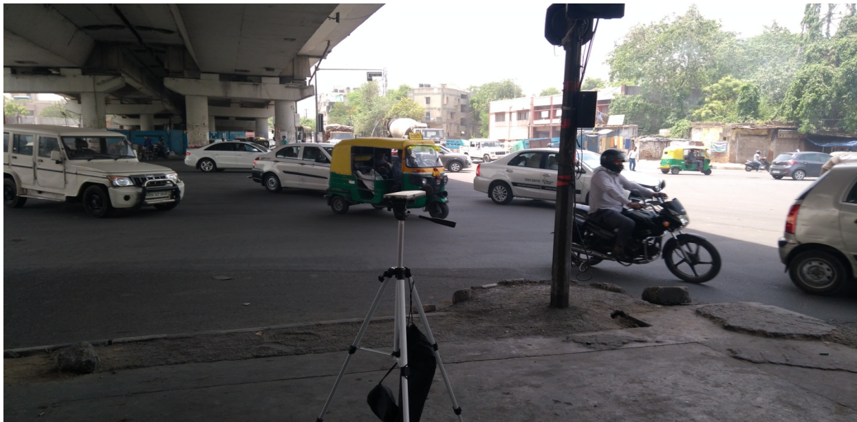
Fig 4.4 Noise monitoring at Ashram Chowk during morning peak time
