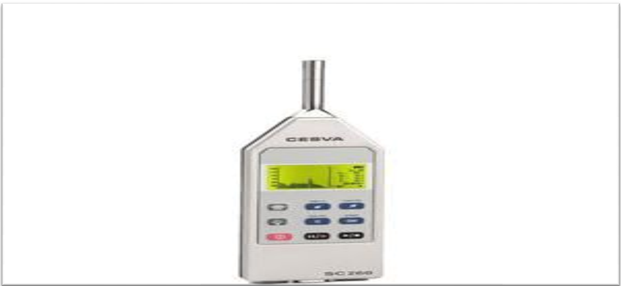
Fig.4.2 Sound level meter
