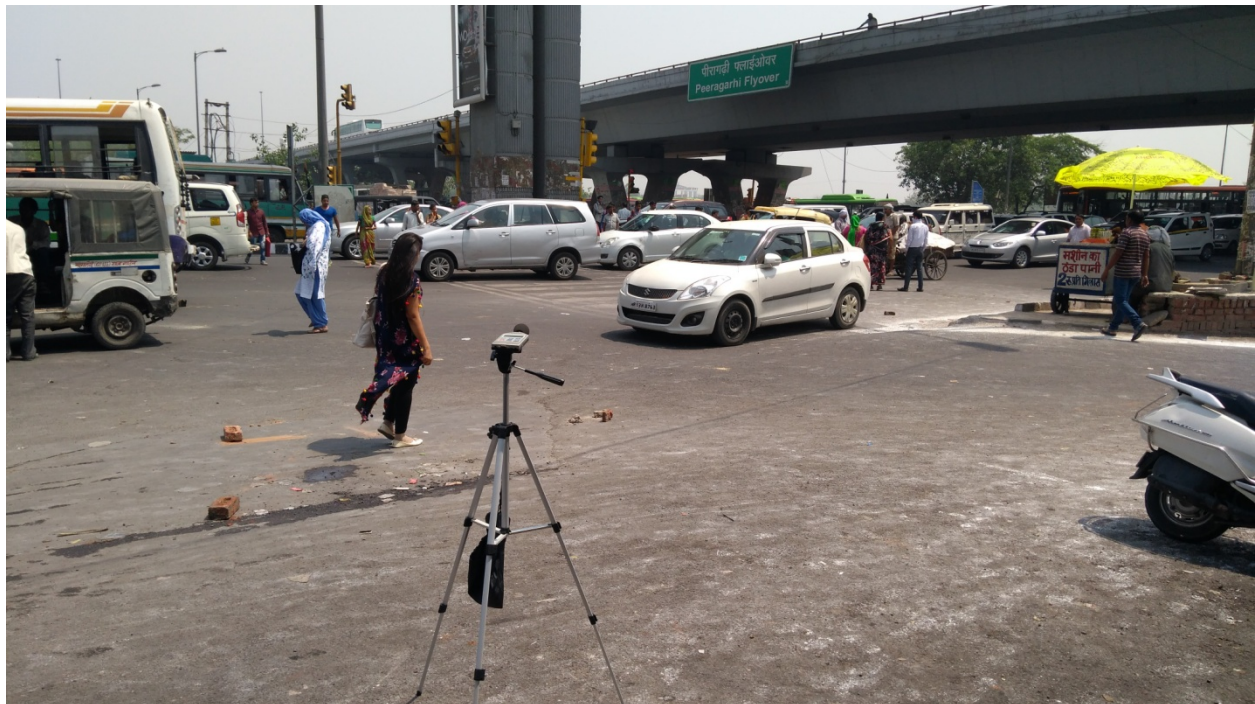
Fig.4.9 Monitoring of the noise level during the morning peak hour
