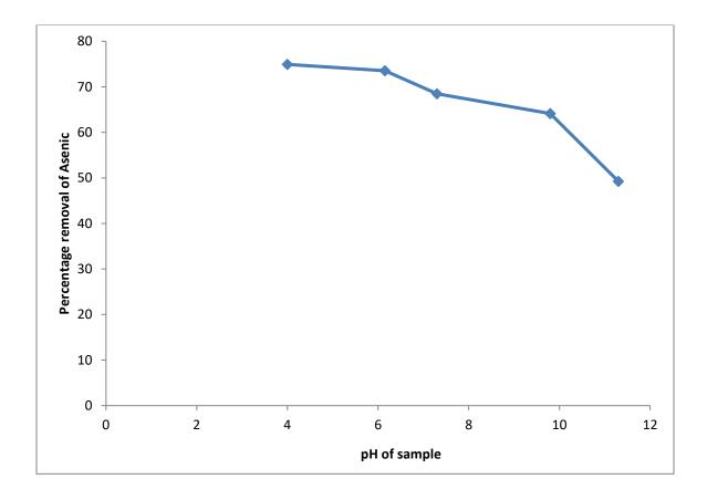
Graph 1 : Percentage removal of Arsenic v/s pH of sample using Coarse Calcite
