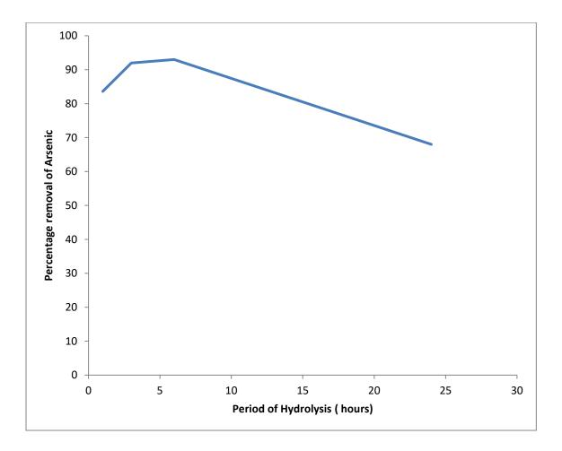
Doping the activated carbon with iron is dependent on the period of hydrolysis. More the hydrolysis period, more will be the doping. But after a certain hydrolysis period, the efficiency reduces significantly. This might be due to the doping capability of the Activated carbon.
