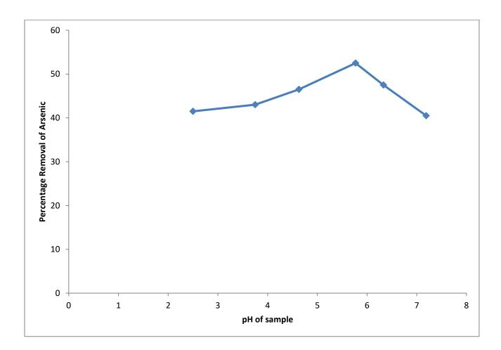
After pH = 2.5 when sodium hydroxide is added, there is an increase in efficiency of removal but it is upto pH = 5.77. But on further addition of sodium hydroxide, the removal efficiency decreases.
