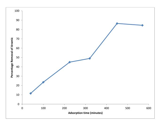
Graph 5: Percentage Removal of arsenic v/s adsorption time using HPPC
