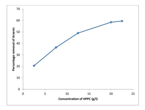
It can be seen that for a particular pH and shaking time the removal efficiency of adsorbent increases with the increase the increase in its concentration.
