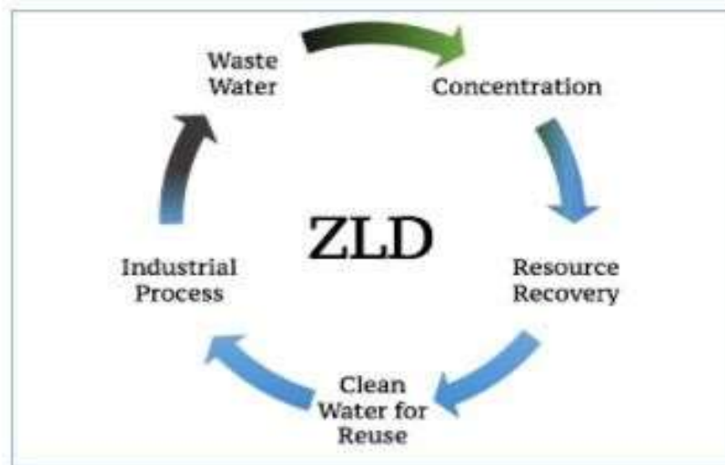
Figure 2.1 Concept of Zero Liquid Discharge
